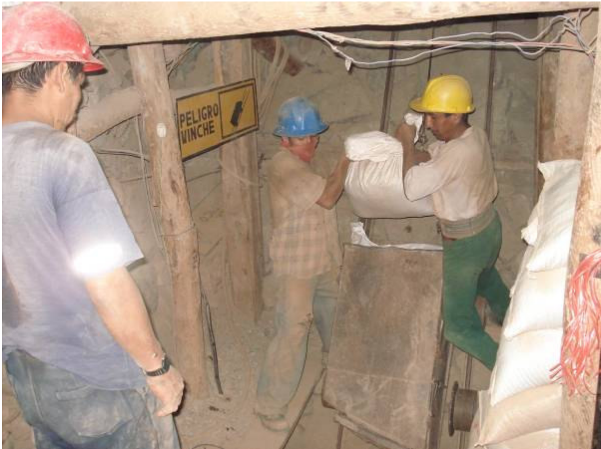
Photo 2: Miners lifting the debris and ore into the trolley. The winche mechanically lifts the trolley out of the mine along a set of rails
