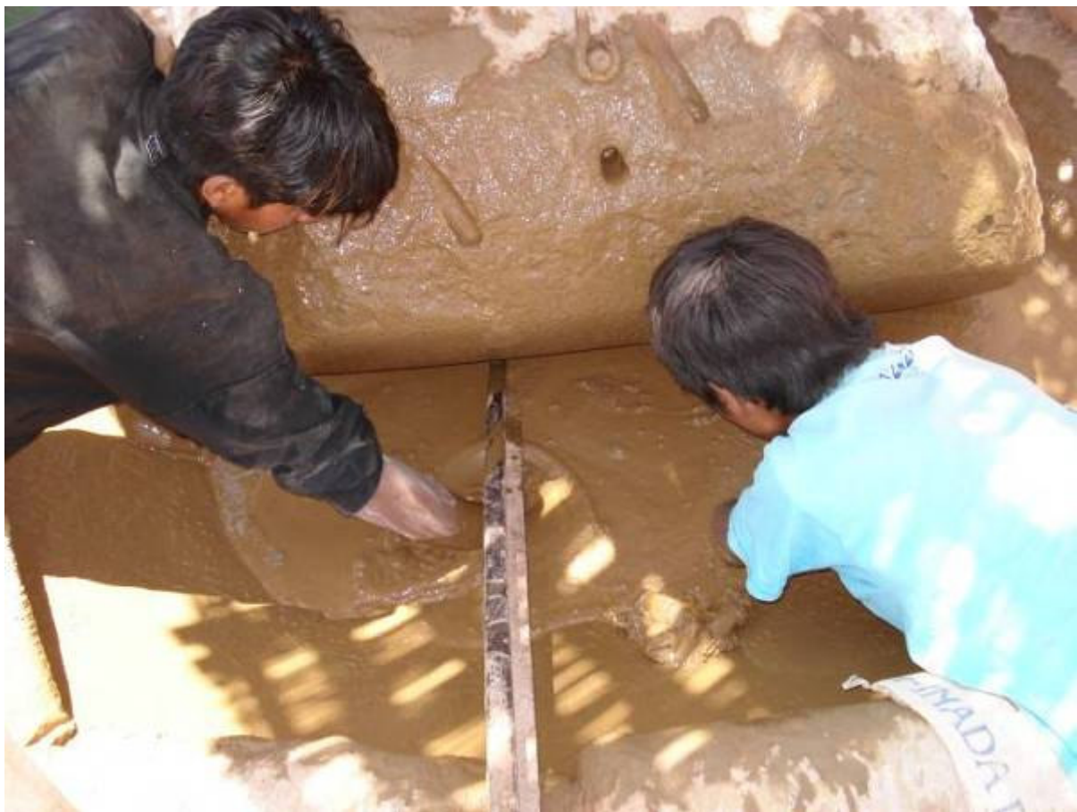
Photo 8: Young boys working the quimbalete; here they are feeling the amalgam to see if it has been sufficiently ground. They do not wear any protective clothing or face masks when handling the mercury mix
